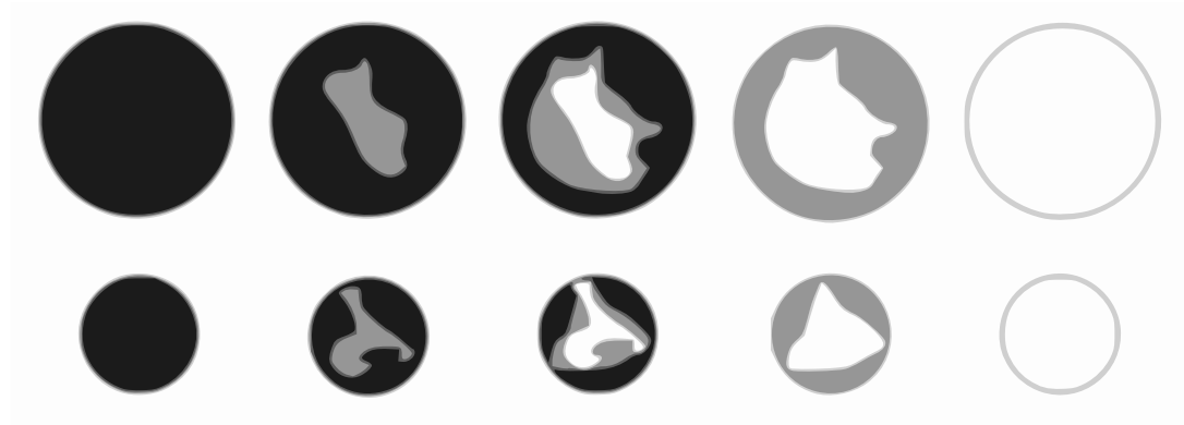
Figure 1.24: Two dimensional representation of the aortic and mitral valves in the model of Schenkel et al. [109]. The black areas represents a no flow boundary, the grey a transition pressure drop (defined by the authors) and the white a zero pressure drop.
