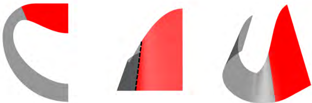
Figure 5.14: Geometry of the growth model with the anterior leaflet highlighted in red with the unmodelled geometry represented in grey. The dashed line in the middle figure shows the line along which the model was constrained in the x-direction. Left – top down view. Middle – front view. Right – three dimensional view.
