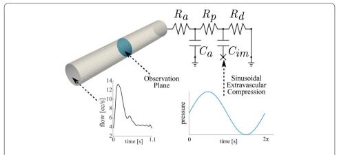
**Fig. 16** Illustration of the problem setup for filtering the five-element coronary LPN using ROUKF-CLS. The inflow velocities are prescribed, and the outflow face is coupled to a Netlist coronary model. The artificial sinusoidal extravascular compression waveform is shown, applied to the base of capacitor  $C_{im}$
