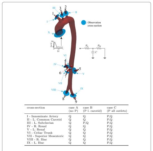
**Fig. 8** Boundary conditions, outlet numbering, and observation planes (depicted in blue, roman numerals) in the subject-specific aorta with synthetic data. The table shows the different sets of observations considered. In all cases, flow was observed at every branch. In case A, no pressure observations were available. Case B used a single pressure observation in the left carotid (outlet III). In Case C, pressure was observed in every branch
