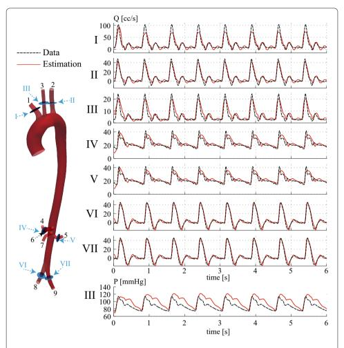
**Fig. 13** Subject-specific aorta with PC-MRI and applanation tonometry data: observations from the model (red lines), computed using the *a posteriori* estimate during the estimation procedure, compared with the measured data (black lines) at each of the seven observation locations for flow, and the location for pressure (outlet III)
