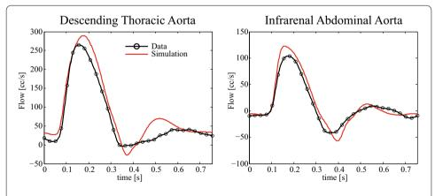
**Fig. 14** Volumetric flow in the descending aorta (left), and the infrarenal abdominal aorta (right) during a forward simulation using the final estimated parameters (see Fig. 12). The waveforms are compared to the PC-MRI data
