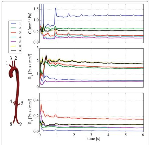
**Fig. 12** Subject-specific aorta with PC-MRI and applanation tonometry data: evolution of Windkessel parameters during estimation for each outlet. Top: compliance C; middle: distal resistance  $R_2$ ; bottom: proximal resistance  $R_1$ . The solid lines denote the estimated values for each parameter; the shaded regions show the range of estimated values plus/minus the the estimation error standard deviation, providing a visual representation of the estimation error
