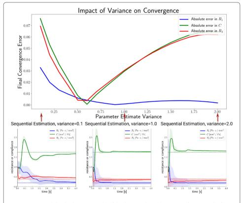
**Fig. 19** Upper panel: the absolute error in each of the three Windkessel parameters after 4 seconds of estimation simulation, at different values of initial parameter estimate covariances  $s_i$  (set uniformly for all three parameters). Lower three images: the parameter convergence history with the initial parameter estimate variances set to 0.1, 1.0 and 2.0 (left to right). See "The choice of initial covariance values for the estimated parameters" section for further discussion
