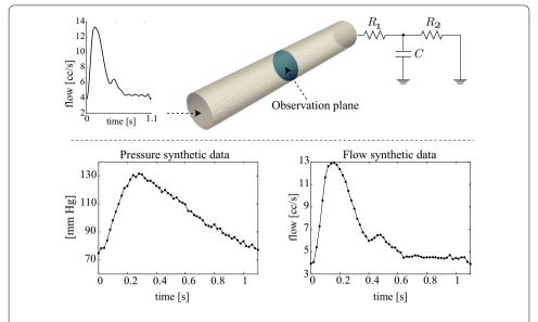
**Fig. 2** Top: problem setup for an idealized carotid artery. The plane where the volumetric flow and cross section-averaged pressure are observed is denoted in blue. The inflow velocities are prescribed using a typical carotid flow waveform and a parabolic velocity profile. The outflow face is coupled to a three-element Windkessel. Bottom: flow and pressure synthetic data (with added Gaussian white noise) created from the mid-vessel observation site during the forward simulation
