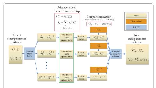
**Fig. 3** Diagram of the estimation procedure during a single time step, showing the interaction between the FSI model and the filtering algorithm. The green box identifies the constrained least squares step, described in "Estimation algorithm—ROUKF-CLS for arbitrary LPNs" section, which is only part of the ROUKF-CLS algorithm (not of the basic ROUKF procedure)
