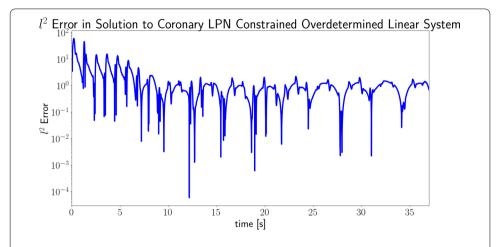
**Fig. 18** Log plot of the  $\ell^2$  norm of the error between the constrained least squares solution and the desired right-hand side for the coronary LPN case, as given by  $\| \mathcal{L}_{LPN}^{over} \mathbf{x} - \mathbf{b} \|$  (cf. Eq. 18). The data is presented over time, demonstrating how the magnitude of the perturbations required to enforce LPN consistency reduces over time, as the parameters converge. The actual parameter values over time for this simulation are shown in Fig. 17
